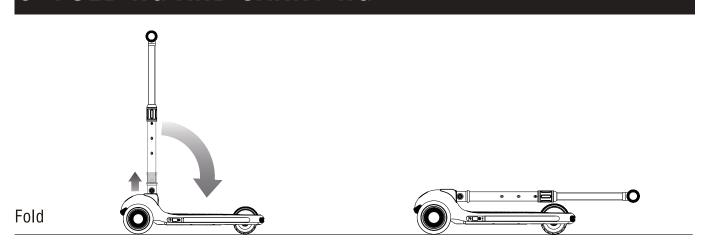
Make sure that the scooter's turned off. Pull up the release sleeve and lower the handlebar stem to fold.
