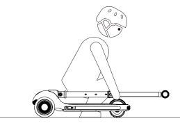
Do not touch the rear fender brake immediately after riding.
