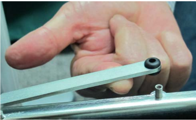
Figure 8-105 Securing the Cage Door with the Securing Arm
