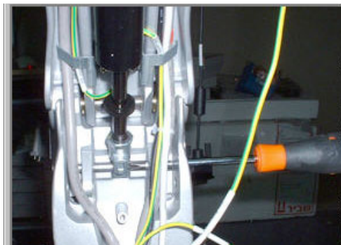
Figure 8-196 Tapping out the Lower Support Pin using a Punch
