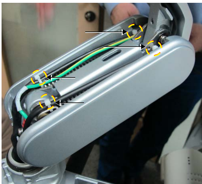
Figure 8-73 Cutting Tie-wraps on the Articulated Arm
