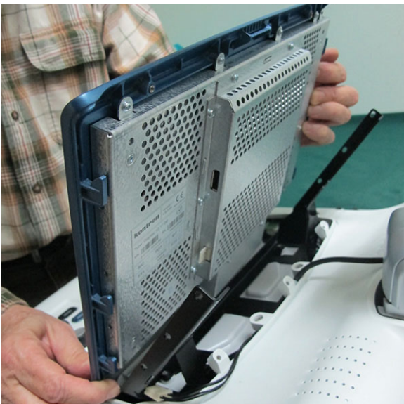
Figure 8-44 Removing the Touch Screen
