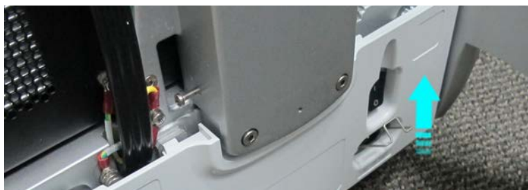
Figure 8-29 Removing the AC Distribution Box Cover
