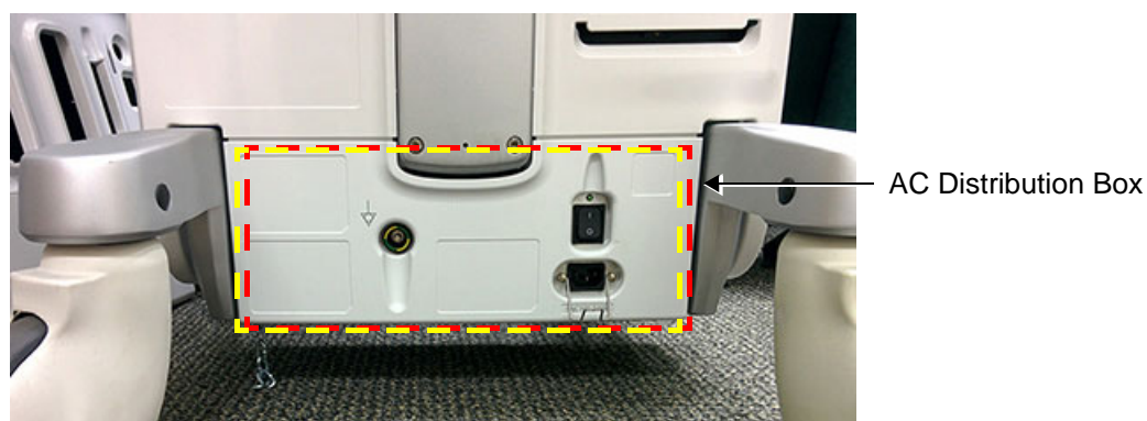
Figure 8-167 AC Distribution Box Located at Rear of System
