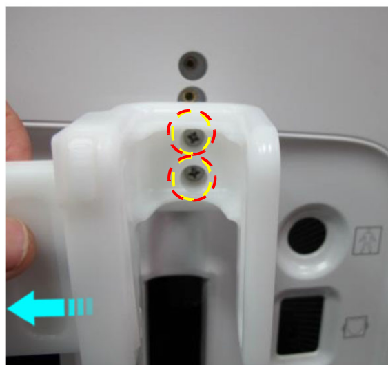
Figure 8-12 Removing the RS Cable Assembly - Front Part
