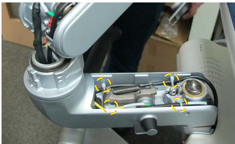
Figure 8-74 Four Tie-wraps on Lower Articulated Arm
