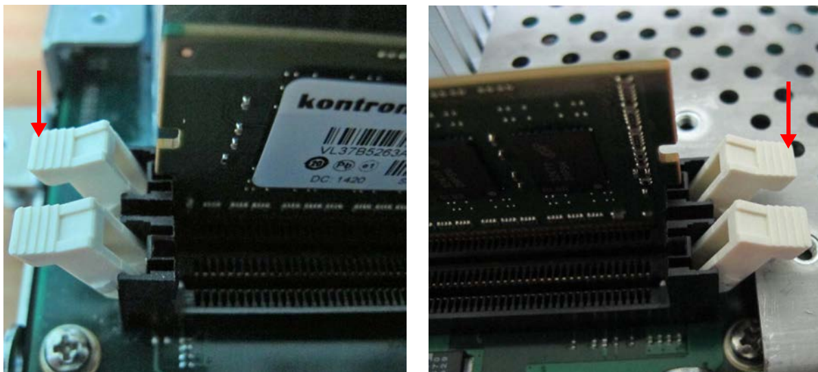
Figure 8-126 Removing the Module Memory DDR Circuit Boards
