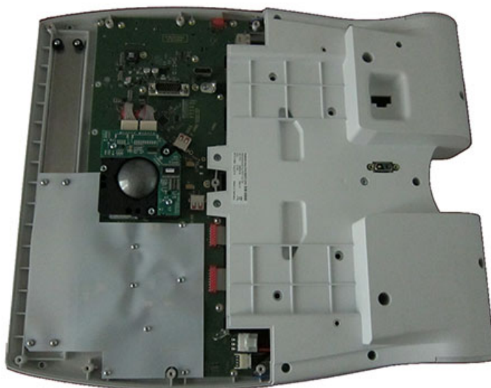
Figure 8-60 Operator Panel Keyboard Assembly with AN Keyboard/Bottom Cover Removed
