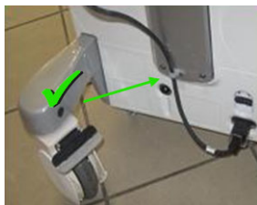
Figure 8-206 AC Power Cable Connected and Routed
