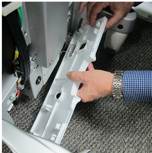
Figure 8-30 Removing the AC Distribution Box Cover
