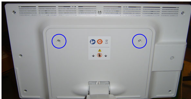
Figure 8-32 Monitor Rear Cover's fixing screws
