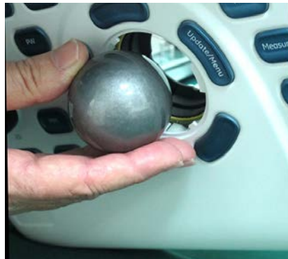
Figure 8-64 Removing the Mechanical Trackball
