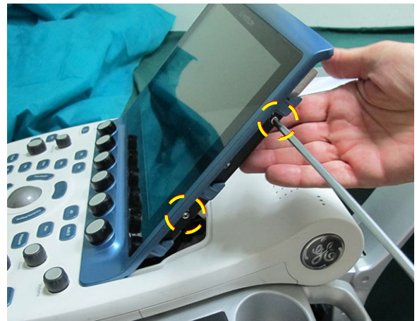
Figure 8-40 Removing the Touch Screen Securing Screws
