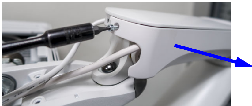
Figure 8-181 Remove the screw and the Upper Service Cover (one side illustrated)
