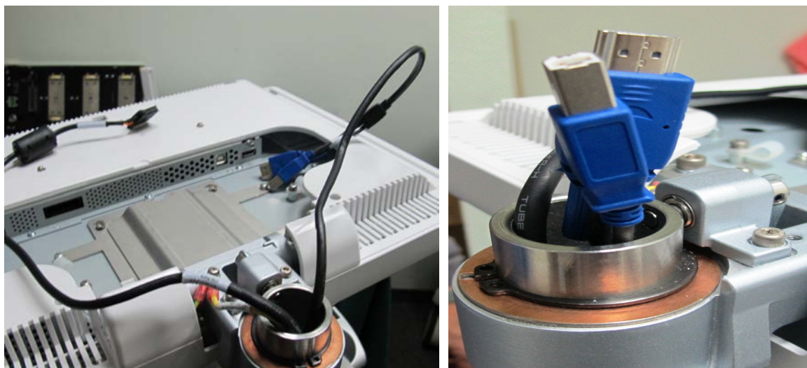
Figure 8-75 Monitor Cables Threaded Through Arm Aperture
