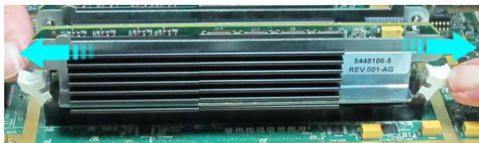
Figure 8-155 Removing a TRX32 Board
