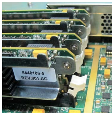
Figure 8-139 TRX32 Boards Secured with Plastic Holders
