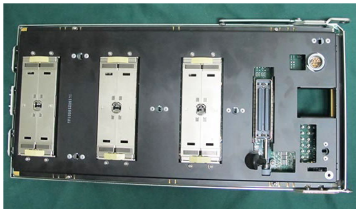
Figure 8-145 Probe Select Board (PSB)
