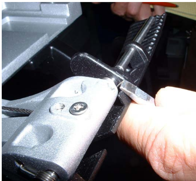
Figure 8-191 Releasing Spring that Presses on the Handle
