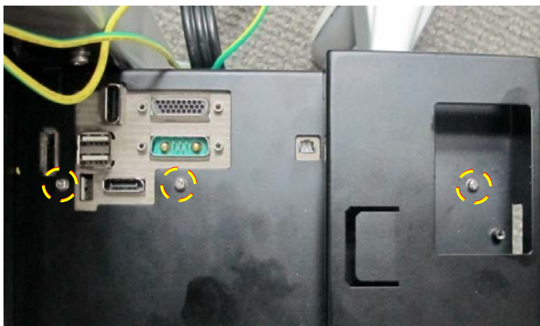
Figure 8-151 BIF Board Securing Screws Located on Top of Cabinet
