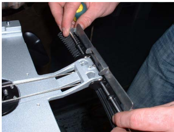
Figure 8-189 Protective Metal Plate Rotated 90 Degrees
