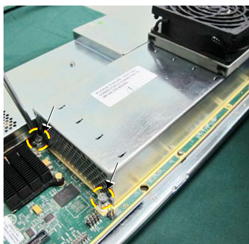
Figure 8-153 Opening the Metal Cover of the TRX32 Box
