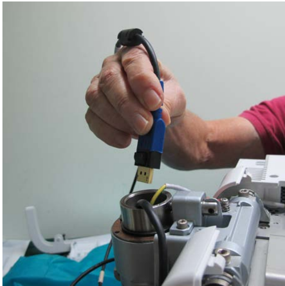
Figure 8-92 Feeding Cables through Top Aperture
