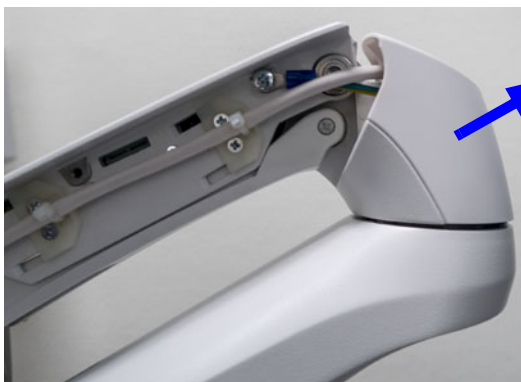
Figure 8-182 Remove the Vertical Service Cover
