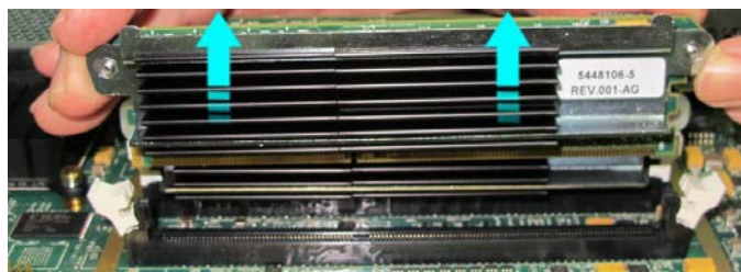
Figure 8-155 Removing a TRX32 Board
