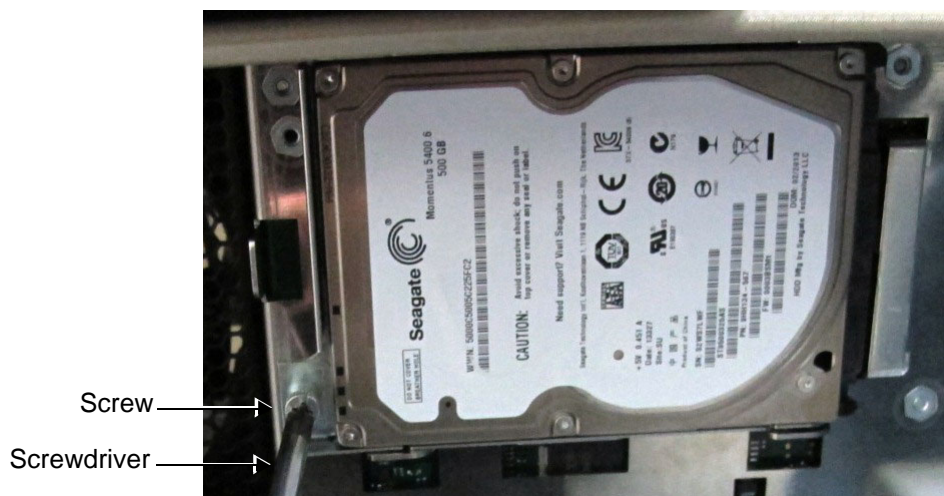
Figure 8-115 Loosening the Screw on the Metal Securing Plate
