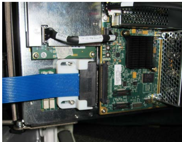
Figure 8-107 Releasing the Retaining Bracket on the CFE
