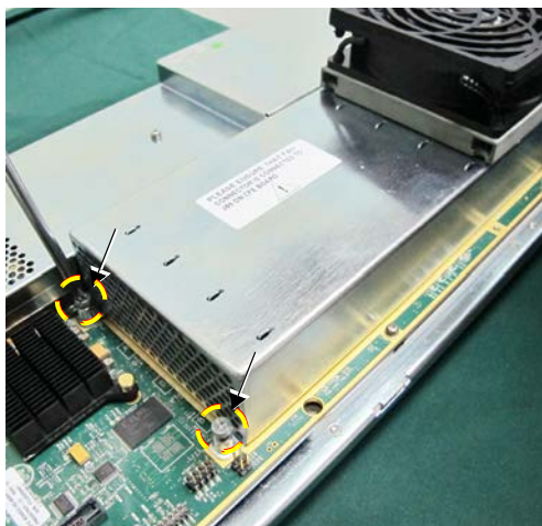
Figure 8-138 Opening the Metal Cover of the TRX32 Box
