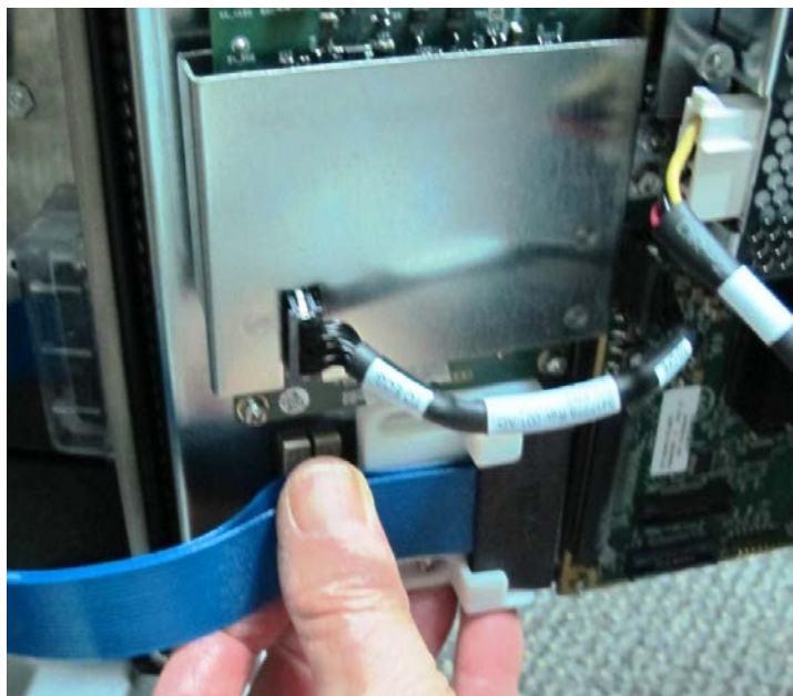
Figure 8-108 Releasing the HDR flat cable from the CFE
