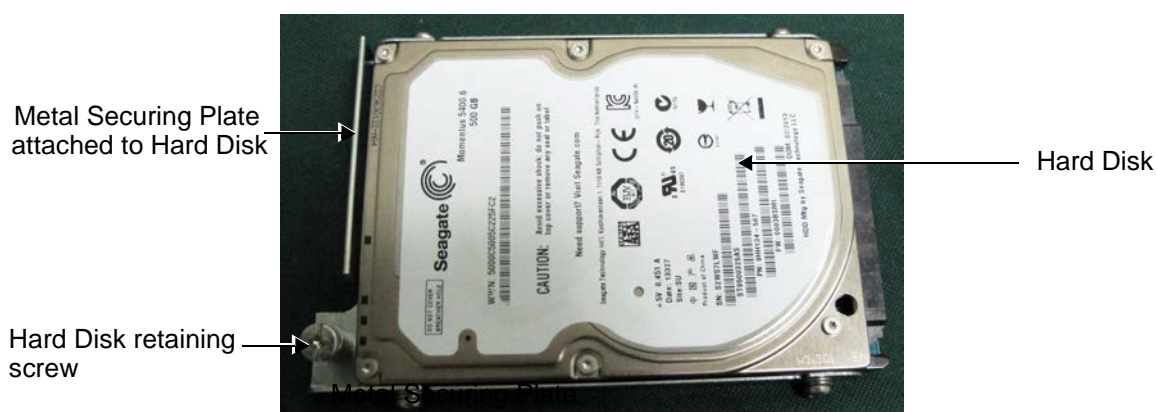
Figure 8-114 Hard Disk with Metal Securing Plate Attached
