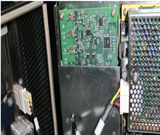
Figure 8-106 Disconnecting BE-to-FEPS Cable from Back End
