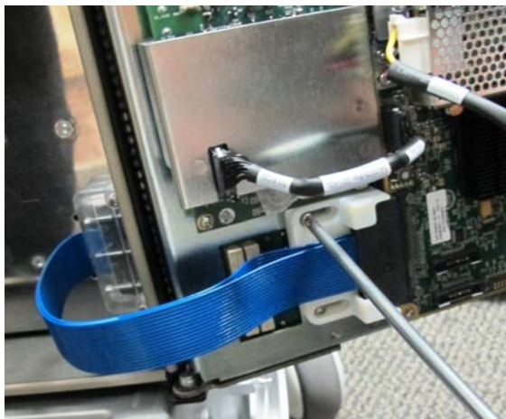
Figure 8-107 Releasing the Retaining Bracket on the CFE
