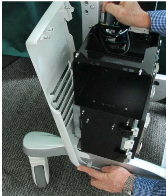
Figure 8-19 Removing the Right Rear Cover
