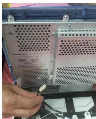
Figure 8-46 Routing and Connecting the Touch Screen Cables
