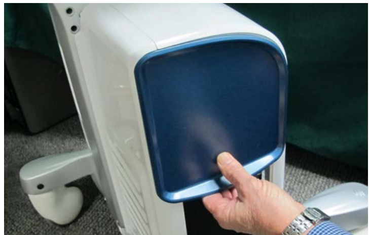
Figure 8-8 Removing the Blank Cover
