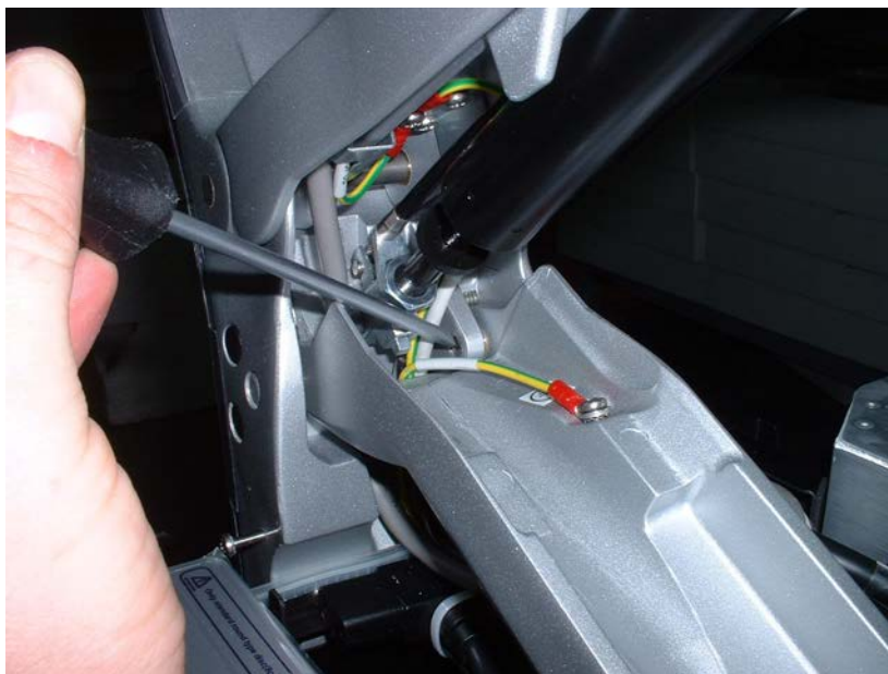
Figure 8-82 Tapping Out the Securing Pin
