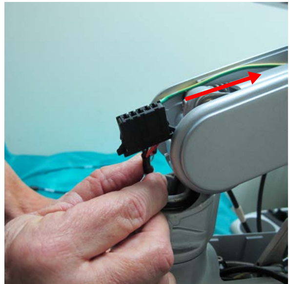
Figure 8-94 Threading the Display to OPIO Cable
