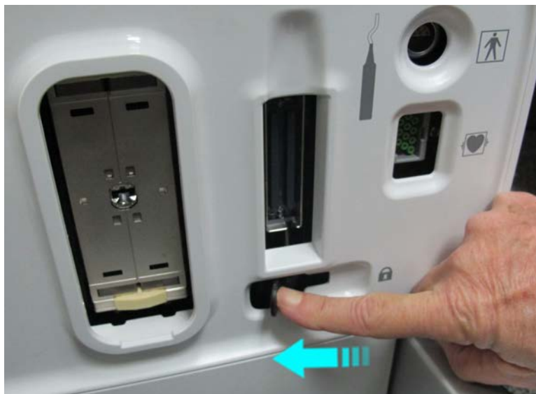
Figure 8-11 RS Probe Connector Lock - OPEN
