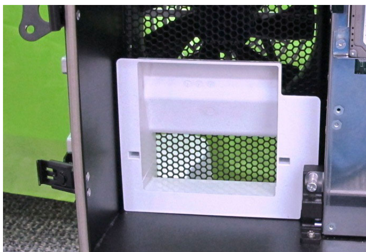
Figure 8-143 Location of Plastic Air Sleeve for CFE
