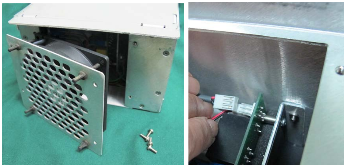
Figure 8-174 Disconnect the Fan Cable from the AC Distribution Box
