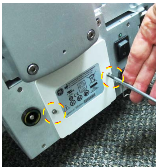
Figure 8-176 Removing the Screw on the Battery Compartment
