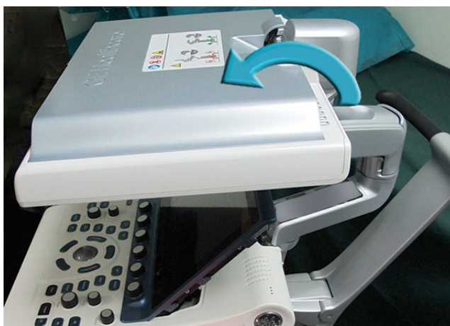
Figure 8-71 Monitor Locked in Face-Down Position
