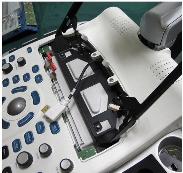
Figure 8-44 Removing the Touch Screen
