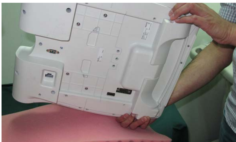
Figure 8-53 Removing the Keyboard Assembly from the System
