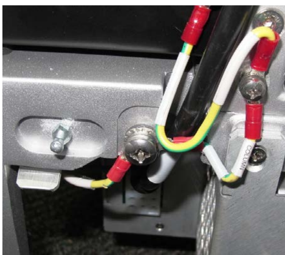
Figure 8-101 Printer-to-AC Box Cable Positioned Behind the Ground Cables
