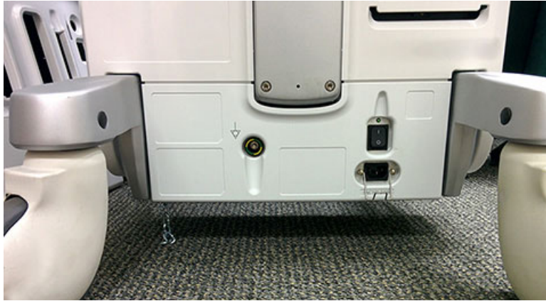
Figure 8-31 AC Distribution Box Cover Installed
