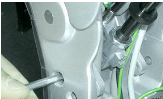
Figure 8-195 Releasing the Securing Screws on Either Side of the Support Arm
