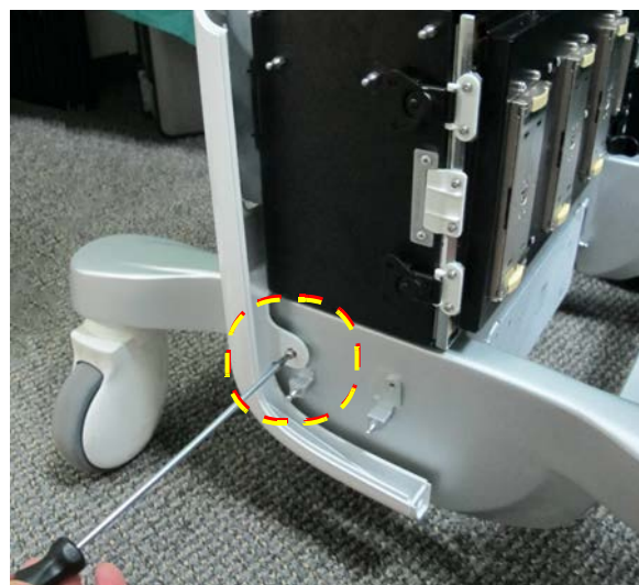
Figure 8-17 Right Rear Cover - Removing Securing Screws
