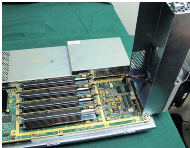
Figure 8-138 Opening the Metal Cover of the TRX32 Box
