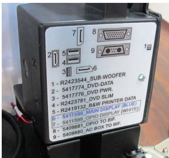
Figure 8-166 Sub-Woofer Showing Location of BIF Connection Map Label
