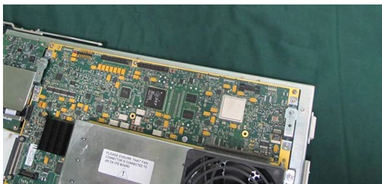
Figure 8-134 Front End Power Supply Removed
