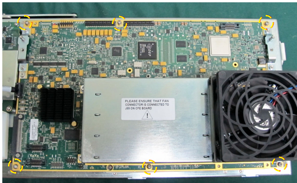
Figure 8-136 CFE Board showing 6 Retaining Screws
