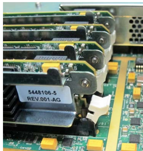
Figure 8-154 TRX32 Boards Secured with Plastic Holders
