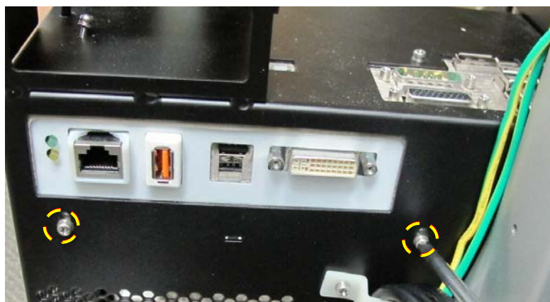
Figure 8-150 Removing the BIF Board Securing Screws Located at Rear of System
