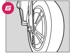
Slide the new motor assembly into the channel on the front forks. Ensure the tire and washers are in the proper position and the tread is facing the correct direction before proceeding. Washers should sit between motor housing and front fork.
