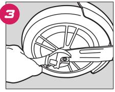
Using a crescent wrench or pair of pliers loosen the nut on each side of the forks.
