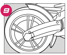
Slide the fork covers back onto the fork and reinstall the 8 screws.
