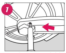
Remove the screws securing the fork covers from the forks. (Keep the screws in a safe place for later use.)
