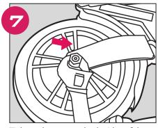
Tighten the nuts on both sides of the forks.
