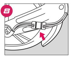
Connect the connectors between the motor and motor adapter.
