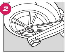
Lift the covers up to remove it off of the front forks.
