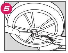
Once the nuts are loosened and the connector has been separated, simply slide the motor assembly down and out of the forks channel.
