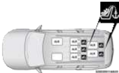
60/40 Second Row (Seven Passenger) Automatic Locking Retractor (ALR) Locations
