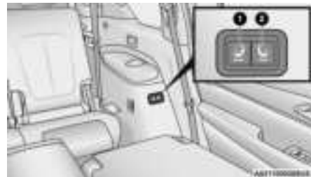
C-Pillar Power Folding Switches (Left Side Shown)
