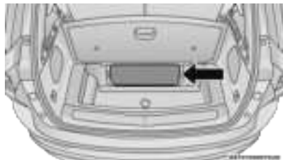
Jack Storage Location (Third Row Seating Without Air Suspension)
