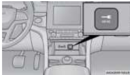
Front Power Outlet
