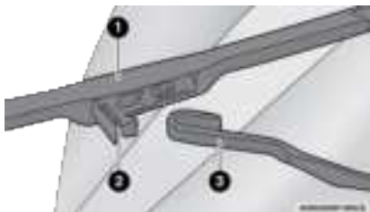
Wiper Blade Removed From Wiper Arm
