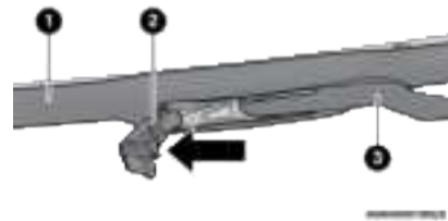
Wiper Blade With Release Tab In Unlocked Position
