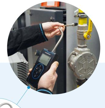
Detect any combustible gas leaks, such as natural gas, methane, propane, isobutane, and LPG, throughout a boiler's gas piping system.
