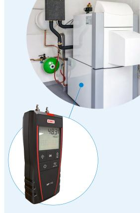
Measure pressure at the gas inlet valve, boiler or furnace draft, and differential pressure across a filter or any other part of the combustion system to verify proper, safe, and efficient operations.
