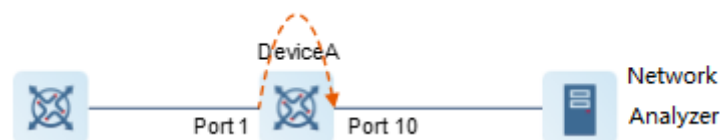
Figure 2-1 Operating Principle of Port Mirroring
