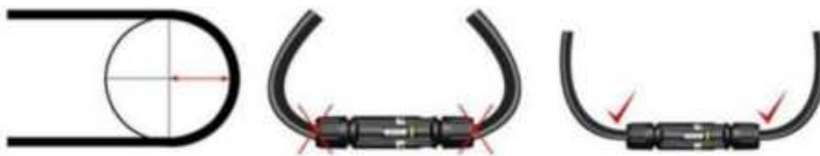
FIGURE 45 MINIMUM BENDING RADIUS OF THE CABLE
