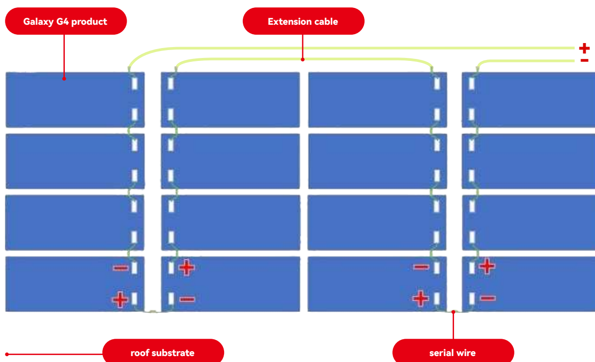
FIGURE 46 PRODUCT JUMPER CONNECTION OPERATION INSTRUCTIONS (FRONT VIEW)
