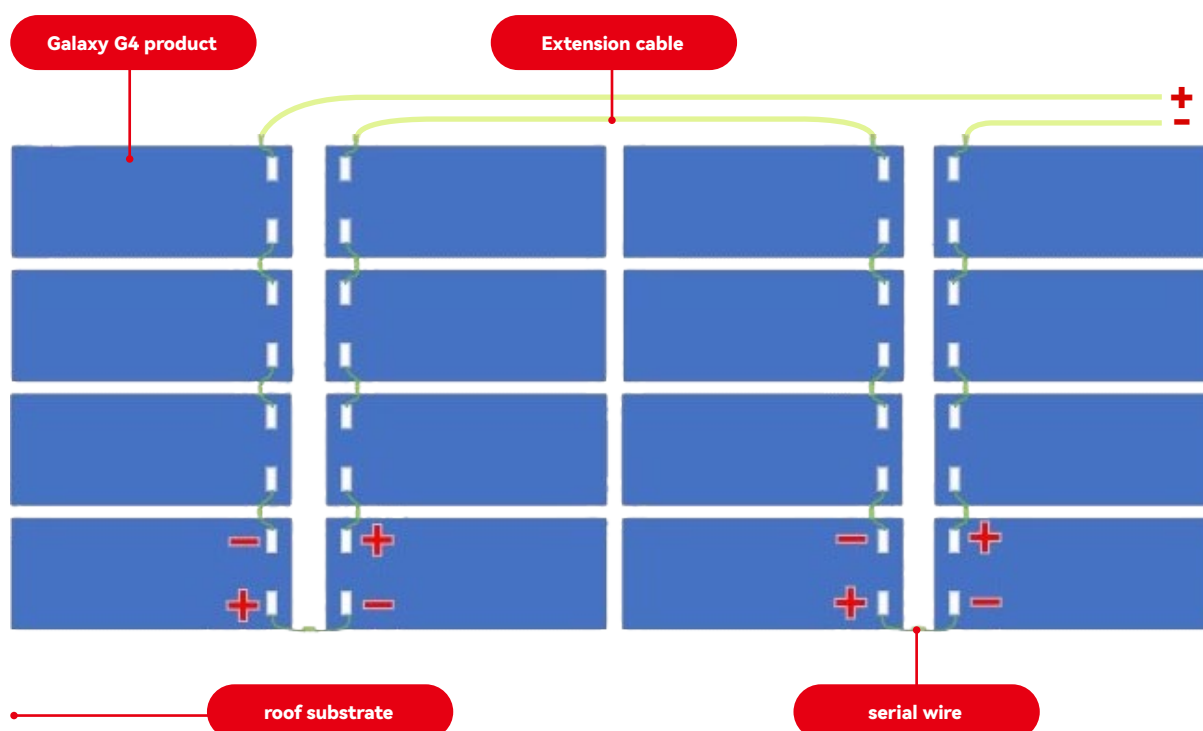
FIGURE 46 PRODUCT JUMPER CONNECTION OPERATION INSTRUCTIONS (FRONT VIEW)
