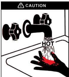
Water temperatures over 125°F can cause severe burns instantly or death scalds. Children, disabled and elderly are at highest risk of being scalded. See instruction manual before setting temperature at water heater. Feel water before bathing or showering. Temperature limiting valves are avaliable, see manual.
