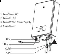
MARNING! If freezing conditions are expected, turn off water and gas and drain all water from the appliance. If power and the automatic frost protection are connected freezing will be prevented.
