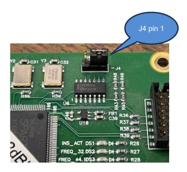
With no input to the AES board the jumper, J4 controls the board's sampling rate. By default the jumper of J4 should be set to pins 1 & 2 (shown) which puts the board in 48kHz mode. DS2 of the AES board will be lit.
