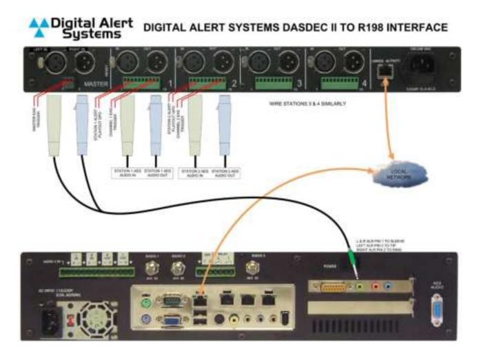
100 to 240 VAC power is input from the universal line in connection. The local ethernet cable RJ45 connector is plugged into the LAN socket.
