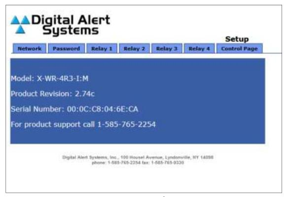
**Setup Configuration** Setup mode of the R198 allows you to customize several settings. Some of the settings are the unit's IP address, Netmask, Gateway, network speed, mode, and passwords.
