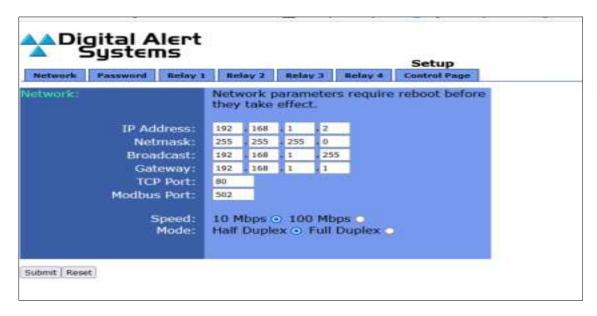
**Permanent storage of IP change** – To store the new Network settings into memory, remove power from the unit, wait approximately 10 seconds, and reconnect power to the unit.
