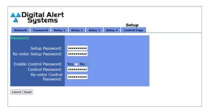
If the passwords are forgotten, the R198 can be set back to factory defaults by removing the power from the unit, pressing and holding, the Reset button on the back of the unit, and reconnecting the power to the unit while keeping the button depressed. After approximately 10 seconds you can release the Reset button and the unit will be reset to the default password of 'digital' for Setup and no password for Control.
