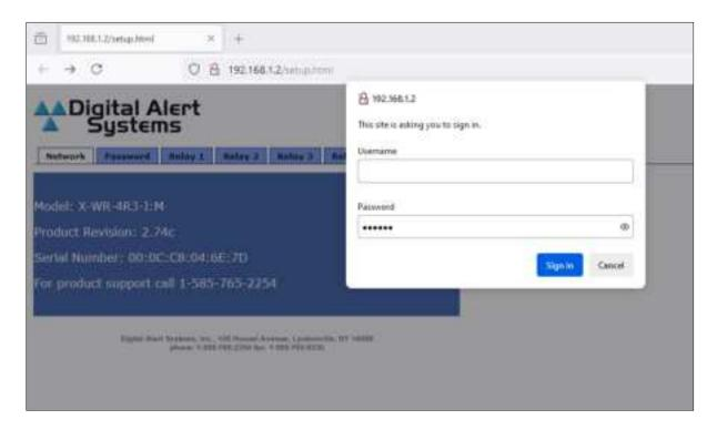
**Changing the Network settings** – Click on the Network tab. Enter the new network settings as desired. After reviewing and verifying your settings, click on 'Submit'. These new changes will show up in the Network tab but will not take effect until the power is removed and reapplied to the unit.
