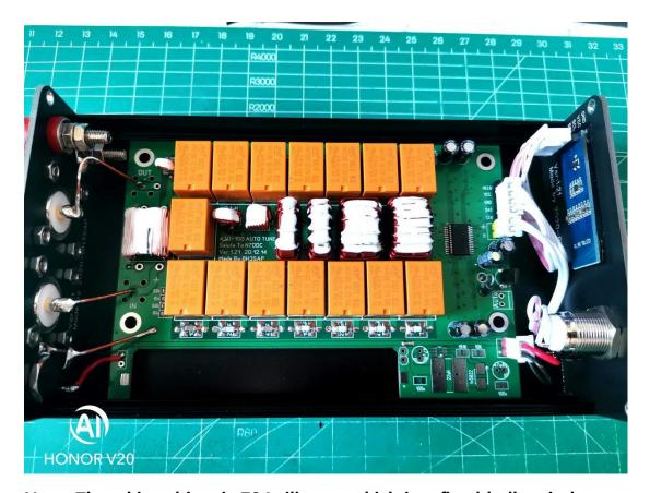
Note: The white object is 704 silicone, which is a fixed hollow inductor and magnetic ring inductor.
