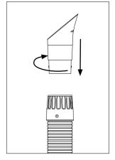
To install a new nozzle, turn the nozzle bayonet clockwise to lock it in place.
