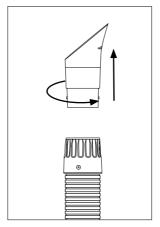
Disassemble the nozzle by holding the tube with one hand. With the other hand turn the nozzle counter-clockwise and pull it out.
