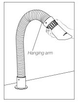
The arm can be used in an upright position with the nozzle hanging over the workplace ...
