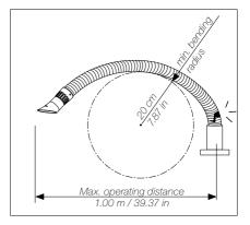
To avoid breaking the arm, do not extend the arm more than 100 cm / 39.37 in from the center of its base and do not go below the minimum bend radius of 20 cm / 7.87 in.
