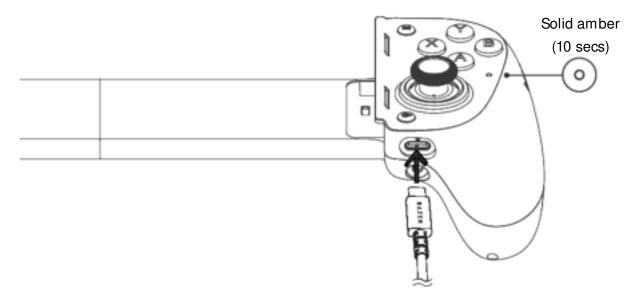
Charging cable not included. Make sure to use only the included USB A to USB C cable. USB Type C audio and other accessories are not supported.
