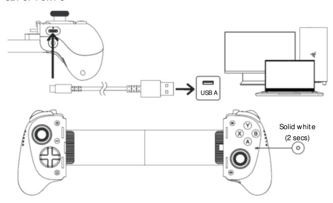
Charging cable not included. Detach your mobile device when using the controller on a PC. The controller will use XInput on Windows.
