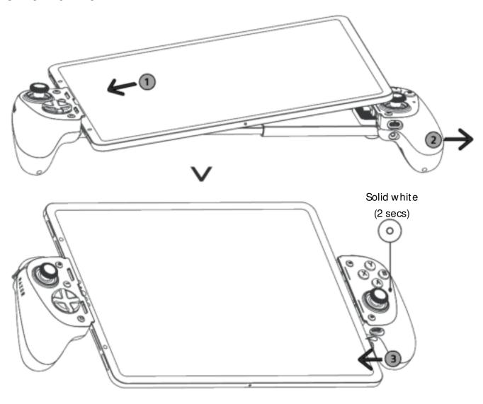
Maximum supported dimensions: 12.32 mm thickness (including camera) x 282 mm length.
