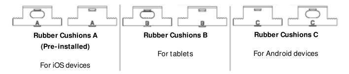
By default, rubber cushions A are pre-installed with the controller. For a case-fitted phone, you can also try removing the rubber cushions to see if it's compatible with the controller.
