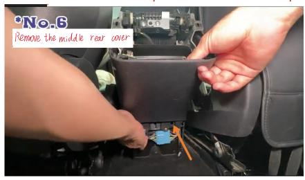
Pull out the original car connector seat
