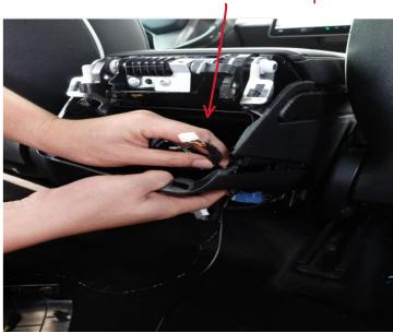
Install the middle of the cover, screw the screw, the cover under the bottom
