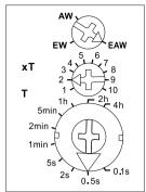
**The LED** below the big rotary switch indicates the contact position while time-out is in progress. It is OFF while the relay contact 15-18 is open (15-16 closed), and is continuously ON as long as the relay contact 15-18 is closed (15-16 open).
