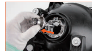
Fig. 1: Remove the dust cover and the OE Halogen bulb. Hold the base of the lamps and turn counter-clockwise until it is unlocked, and then remove the OE Halogen bulb;
