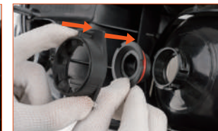
Fig. 2: Assemble the retainer holder with the bulb retainer together, and then insert them into the assembly.
