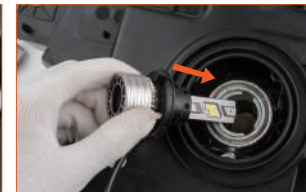
Fig. 2: Insert 9008/H13 into the assembly and rotate it clockwise, then lock it.
