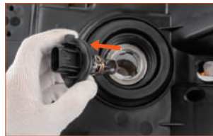
Fig. 1: Remove the OE halogen bulb.
