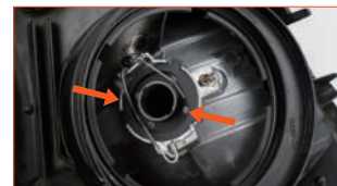
Fig. 2: Insert the retainer holder into the assembly slot, match the tabs with slot, and lock the retainer holder with the buckle;
