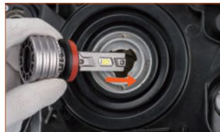
Fig. 2: Line-up the tabs with the slots of the assembly. Warn: the tabs are asymmetrical.
