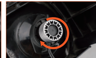
Fig. 4: Rotate the heat sink to make it tight (If the high beam and the low beam reverse, take the bulb out and rotate it 180 degree, and then install it again.)
