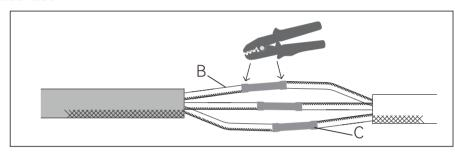
3. Winding the waterproof electrical tape on the butt splice connections of three strands of wire.
