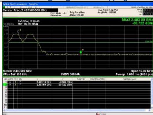
Out Of Band Emission(Right) GFSK_DH5_Channel Hopping
