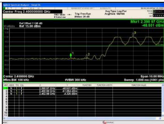
Out Of Band Emission(Left) GFSK_DH5_Channel Hopping
