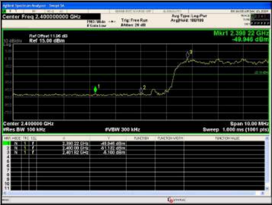
Out Of Band Emission(Left) 8DPSK_3-DH5_Channel Hopping
