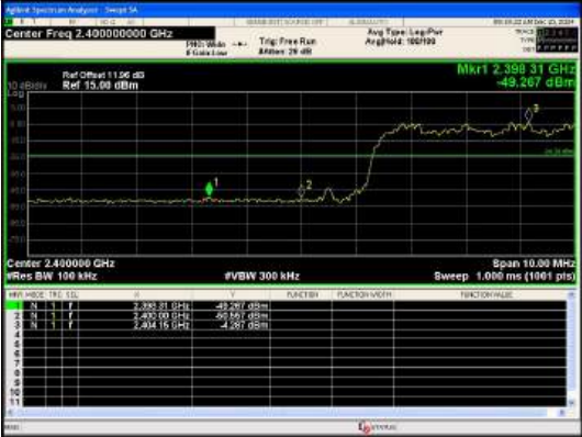
Out Of Band Emission(Left) 8DPSK_3-DH5_Channel Hopping
