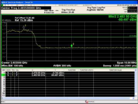
Out Of Band Emission(Right) 8DPSK_3-DH5_Channel Hopping
