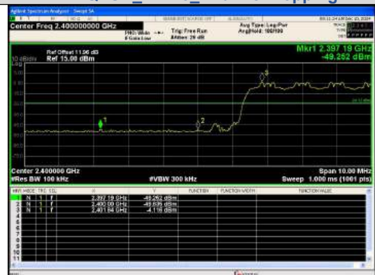
Out Of Band Emission(Left) \pi/4 DQPSK_2-DH5_Channel Hopping
