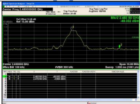
Out Of Band Emission GFSK_DH5_Channel 78
