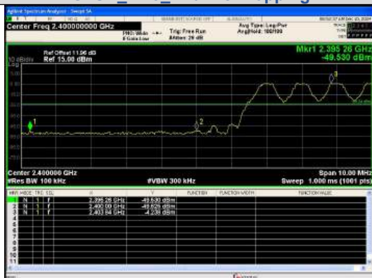
Out Of Band Emission(Left) GFSK_DH5_Channel Hopping
