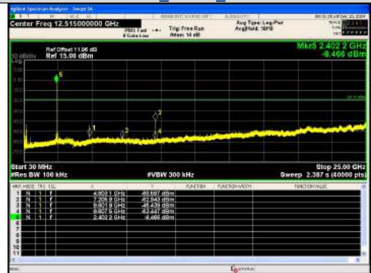
30.0 MHz - 25000.0 MHz \pi/4 DQPSK_2-DH5_Channel 0
