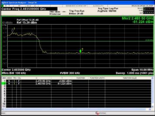
Out Of Band Emission(Right) 8DPSK_3-DH5_Channel Hopping
