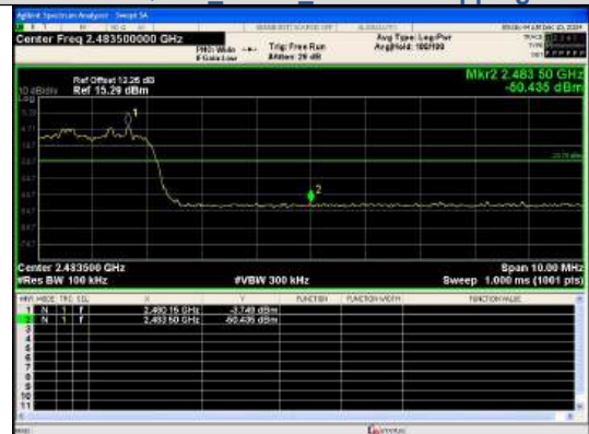
Out Of Band Emission(Right) \pi/4 DQPSK_2-DH5_Channel Hopping
