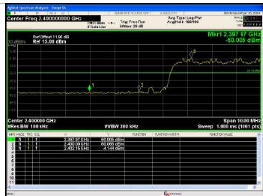
Out Of Band Emission(Left) \pi/4 DQPSK_2-DH5_Channel Hopping
