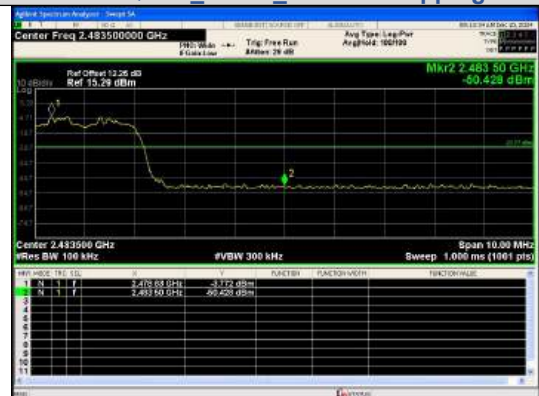
Out Of Band Emission(Right) \pi/4 DQPSK_2-DH5_Channel Hopping
