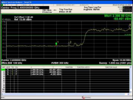
Out Of Band Emission(Left) 8DPSK_3-DH5_Channel Hopping
