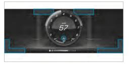
If you select the progressive display setting in vehicles with a Widescreen Cockpit, the position of the indicator lamps in the Instrument Display changes.
