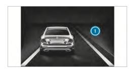
If a lane-correcting brake application occurs, display 1 appears in the multifunction display.
