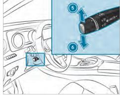
Press the lever briefly: stored speed is increased (a) or reduced (b) by 1 km/h.
