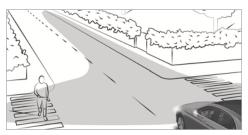
Cornering light improves the illumination of the carriageway over a wide angle in the turning direction, enabling better visibility in tight bends, for example. It can only be activated when the dipped beam is switched on.
