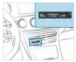
When the ignition is switched on, a system selftest is performed during which the two PASSENGER AIR BAG ON and OFF indicator lamps light up simultaneously.
