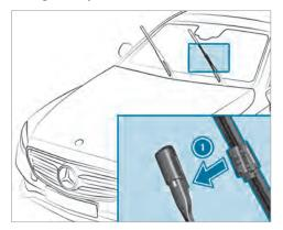
Insert the new wiper blade into the wiper arm in the direction of arrow ①.
