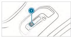
Switches the reading lamp on/off
