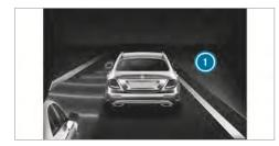
If a course-correcting brake application occurs, the red warning lamp flashes in the outside mirror and a warning tone sounds. In addition, a display 1 indicating the danger of a side collision appears in the multifunction display.
