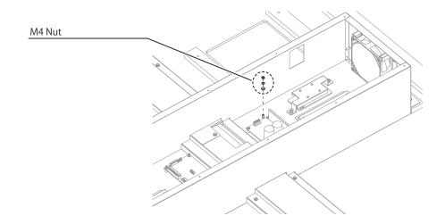
Replace the Air Gimmick Box on the Roof Base.
