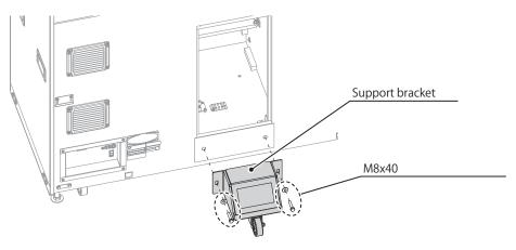
Attach the Support Bracket inside the Cabinet with 2 hex bolts.
