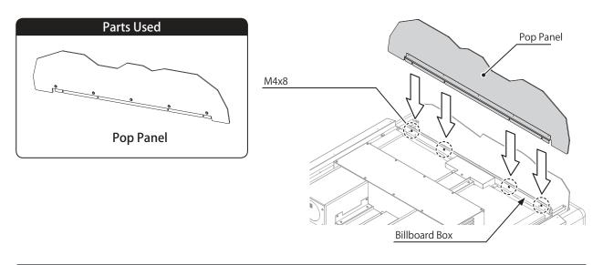
**9** Fully tighten the four screws used in step 1.
