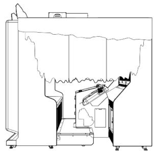
FIG. 7-1b Separate components when moving over a sloped or stepped area.
