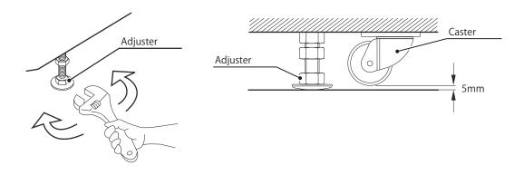
After adjustment, tighten the nut of the adjuster upward and fix the height of the adjuster.
