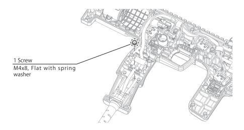
Lift the Controller cable and disconnect connector
