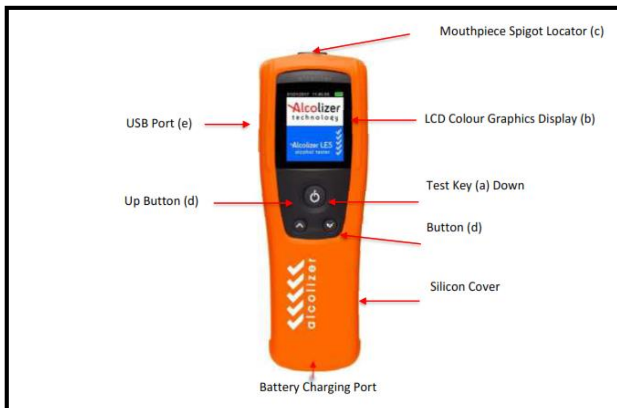
Figure 1 User Display, Buttons and Adapter Sockets
