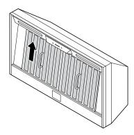
Pull the bottom of the filter forward and remove it.
