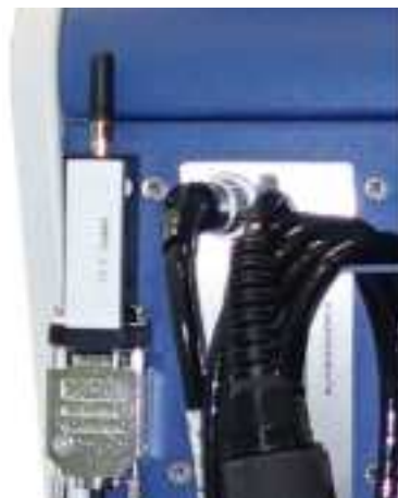
Fig. 21: Fasten the transmitter with Velcro in a free place
