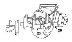
Run the float wheel with only 4 to 5 pounds of pressure during operation. Plant spacing can be changed slightly by increasing or decreasing the tire pressure.
