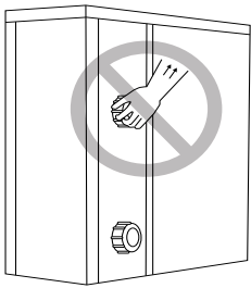
Do not lift the water union as you may damage the heat exchanger
