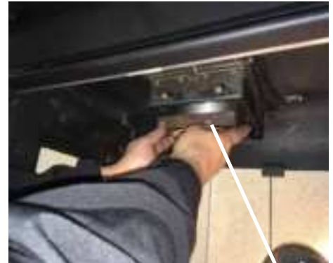
Install square support and catalyst into cartridge
