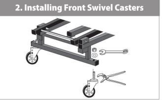
Attach front swivel casters as shown. While tightening nuts, grip bearing cap with channel lock pliers or pipe wrench to prevent threaded stem from turning. Tighten nuts firmly but not excessively. Check nut tightness on caster stems periodically.
