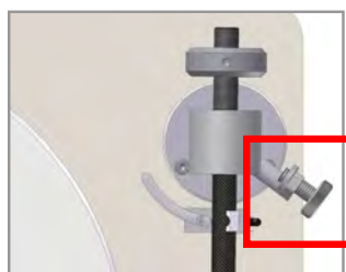
Illustration 1 : Minimal antiskating (Screw is almost removed)
