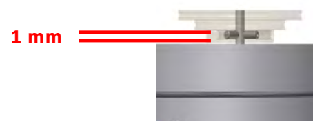
Pic. 12: Mounting the pulley
