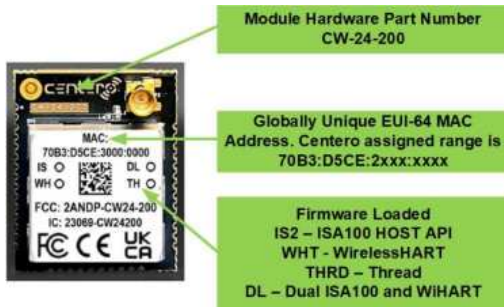
Figure 2 – WIHART2/WISA2 Module Markings
