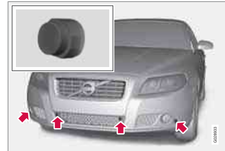
Location of the front sensors
