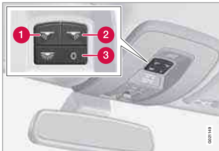
Light switches, front roof lighting
