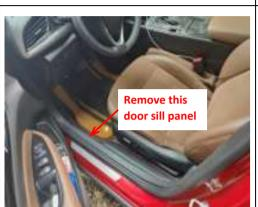
3. Remove the front left door sill panel and lift up the floor mat to find out the fuse box.
