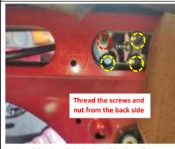
16. Thread the three bolts(indicated by the yellow circles) through the bracket from the back side, use nuts to secure them and use another nut to secure the countersunk screw.
