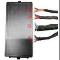
31. Insert the left and right strut wire harnesses (1)(2), lock signal harness (3), and power harness (4) into the ECU in sequence.
