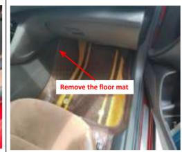
5. Remove the floor mat from the front passenger's position.
