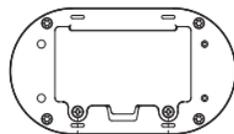
Two screws securing batteries
