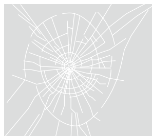
< Broken Laminated Glass >
