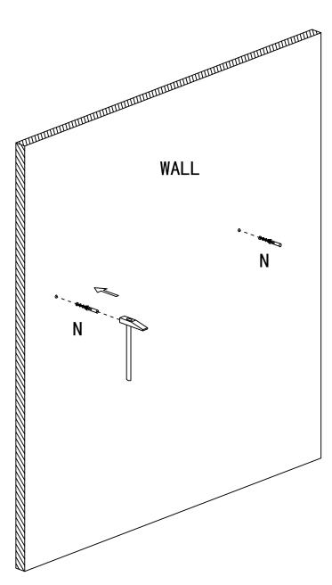
$\phi 8\text{mm}$  hole on the wall, depth 50mm
