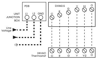
Digital 2 Heat, 2 Cool, MCO, or ACO provides auto speed change (for CXM2 connect Y2 to blower relay coil - see the wiring diagram).
