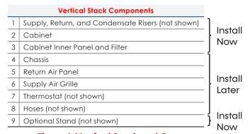
Figure 1: Vertical Stack and Components
