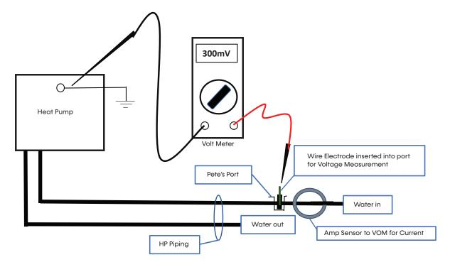
Measure the electrolysis voltage using a volt meter between the heat pump ground and a #14 AWG solid copper wire electrode inserted into the water using a Pete's style access port.
