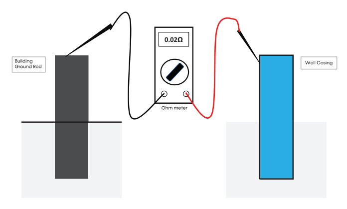
Measure the earth ground bond using an Ohm meter between the building's ground rod and the steel well casing.
