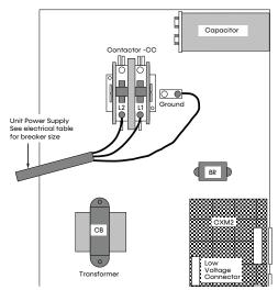
NOTE: 460V units with an EC motor or Internal Secondary Pump require a neutral wire. Three-phase wiring is similar except that all three power wires are directly connected to the contactor.
