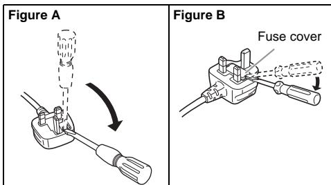
2. Replace the fuse and close or attach the fuse cover.
