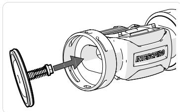
6. Put the exhalation valve cover back onto the adapter.
