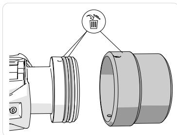
9. Lubricate two new O-rings with silicone lubricant and put them on the filter adapter.
