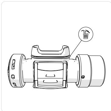
2. Lubricate a new O-ring with silicone lubricant and put it on the filter adapter.
