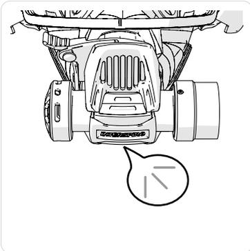
2. Make sure the adapter is mounted so that the text INTERSPIRO is readable from the front of the mask.
