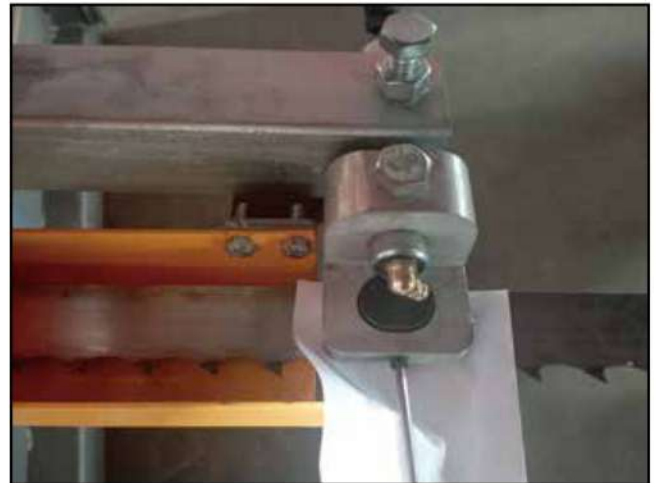
Adjusting the gap above the saw blade.
