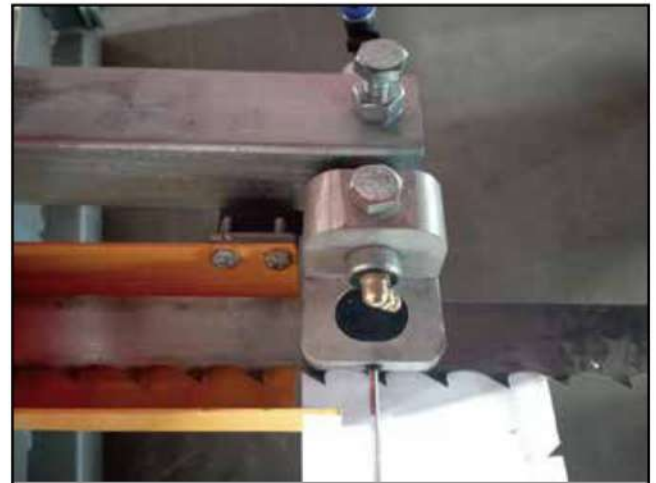
Adjust the gap below the saw blade.
