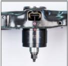
Place the housing 4925-58 with the pre-centred lower silent block, the installation/removal disc 4925-61 and the distance pipe 4925-64 onto the unit support and then screw on the spindle nut 4925-11 until a frictional connection is made.
