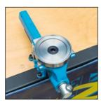
• Clamp the vice adapter 4925-60 in a vice and fit the housing cover 4925-59 and the housing 4925-58.
