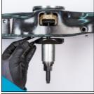
• Then fully insert the lower silent block.
