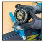
Actuate the spindle nut 4925-11 using a ratcheting combination wrench 606-24, while at the same time holding up the threaded spindle 4925-67 using a double box-end wrench 630-10x11 and insert the upper silent block completely into the housing 4925-58.
