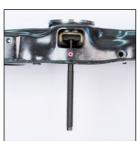
• Screw spindle 4925-67 into the centring disc.
