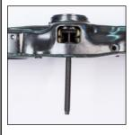
Screw the threaded spindle 4925-67 through the bearing with the installation/removal disc 4925-61.
