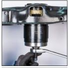
Actuate the spindle nut 4925-11 using a ratcheting combination wrench 606-24, while at the same time holding up the threaded spindle 4925-67 using a double box-end wrench 630-10x11, until the silent block is completely exposed.
