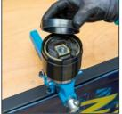
Screw in the threaded spindle 4925-67 and place the spacer ring 4925-62 on top of it. Then place the installation/removal disc 4925-61 over it.
