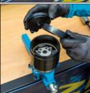
• Then remove the spacer ring 4925-62 and turn over the installation/removal disc 4925-61.
