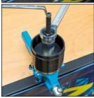
• Then fully insert the lower silent block by actuating the spindle nut 4925-11 using the ratcheting combination wrench 606-24, while at the same time holding up the threaded spindle 4925-67 using a double box-end wrench 630-10x11.
