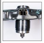
Then screw the housing 4925-58 and housing cover 4925-59 with the spindle nut 4925-11 onto the threaded spindle 4925-67.
