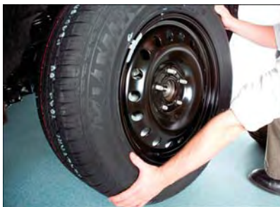
Installing Spare Wheel/Tire
