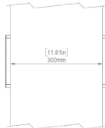
Fig. 5 - Example 2: installation of 2 readers on each side of a wall
