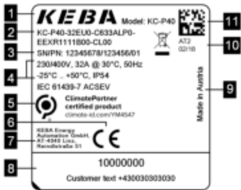
1 ... Manufacturer 2 ... Product key 3 ... Serial number / Material number 4 ... Electrical data 5 ... ClimatePartner certification 6 ... CE marking 7 ... Manufacturer address 8 ... Operator information 9 ... Country of manufacture 10 ... Production location and date 11 ... Production code
