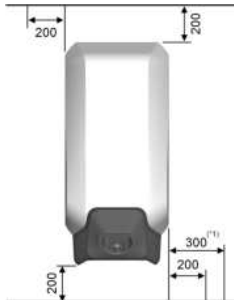
Fig. 8-1: Minimum distances in millimetres
