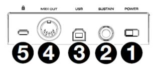
2. Sustain Pedal Input: This input accepts a momentary- contact foot pedal (not included). When pressed, the pedal by default will sustain the sound you are playing without you having to keep your fingers pressed down on 5 4 3 2 1 the keys. The sustain pedal input can be remapped to perform a custom MIDI assignment.
