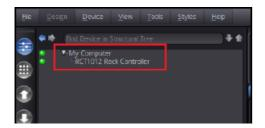
**Note:** If the RCT 1012 does not appear on the APPolo Control GUI as indicated above, check your USB connection and verify if the device is detected in the PC device panel. If the USB connection is made correctly and the device is still not detected, restart APPolo Control GUI.
