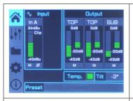
On the main screen you can see the cabinet's input and output.
