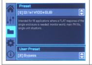
The folder screen shows you the name of the preset and its description. Using the joystick you can change the preset.
