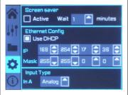
This screen is to configurate Ethernet. You can choose automatic or manual You can also configure the screen saver.
