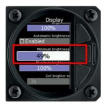
With a push of the middle button, you can activate the slide control, and then by pushing the top and bottom buttons you can select the preferred value and confirm it via the middle button.
