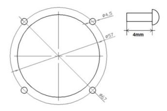
**WARNING:** The length of the screw is limited to a maximum of 4mm!
