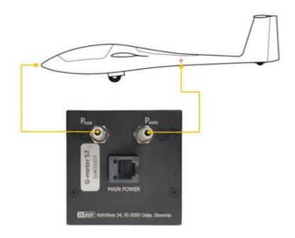
**WARNING:** Static ports are used for flight loggers. Without static ports connected device will still have all other functionalities.
