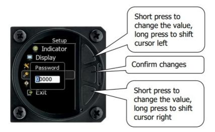
Once the required value is selected, long press the lower push button to move to the next character selection. To move back to the previous character, long press the upper push button. When you have finished editing press the middle push button. A long press of the middle push button exits from the edited field ("control") without any changes.
