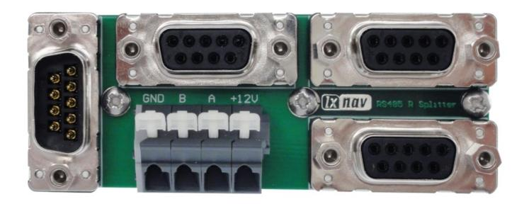
After that small modification, fixing the Bridge to the RS485 splitter will be very easy. On the other side of the Bridge there is a RJ12 connector with a standard IGC/FLARM pinout
