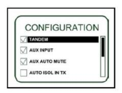
Try to enable "Tandem" mode on the radio itself. To do this, press MDE while turning on the radio. Input password 6435 and press STO. Move to "Configuration" screen with SCN and enable "Tandem" checkbox there. Also, on the "SPKR VOL SRC" select the "Both" option. Now you can turn off the radio (settings are saved on-the-fly) and check if the connection works. If it still doesn't work or you can't find the menu items, please specify the exact model of Becker radio (the "PN" label on the device).
