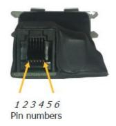
On the other side of the Bridge there is a RJ12 connector with a standard IGC/FLARM pinout
