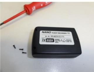
• Open the cover and remove the battery:
