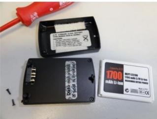
• Insert a new Nokia 3310 battery (Li-Ion). Make sure that the contacts are properly aligned. Close the cover and carefully screw back the three screws:
